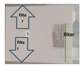
1. The filter on the side of the evaporator (air inlet): Unscrew the two self-tapping screws on the box cover, pull it out, rinse it with clean water, and dry it before putting it back.
